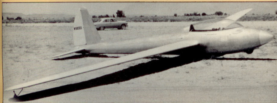
A change to tandem seating made a fine sailplane of the Hummingbird, after which it was redesigned in metal. Empty, the nose wheel is off the ground. Rollers under the wingtips permit taxiing with one wing down. A closeup of an occupied Hummingbird shows the side-hinged canopy and the engine extended.
