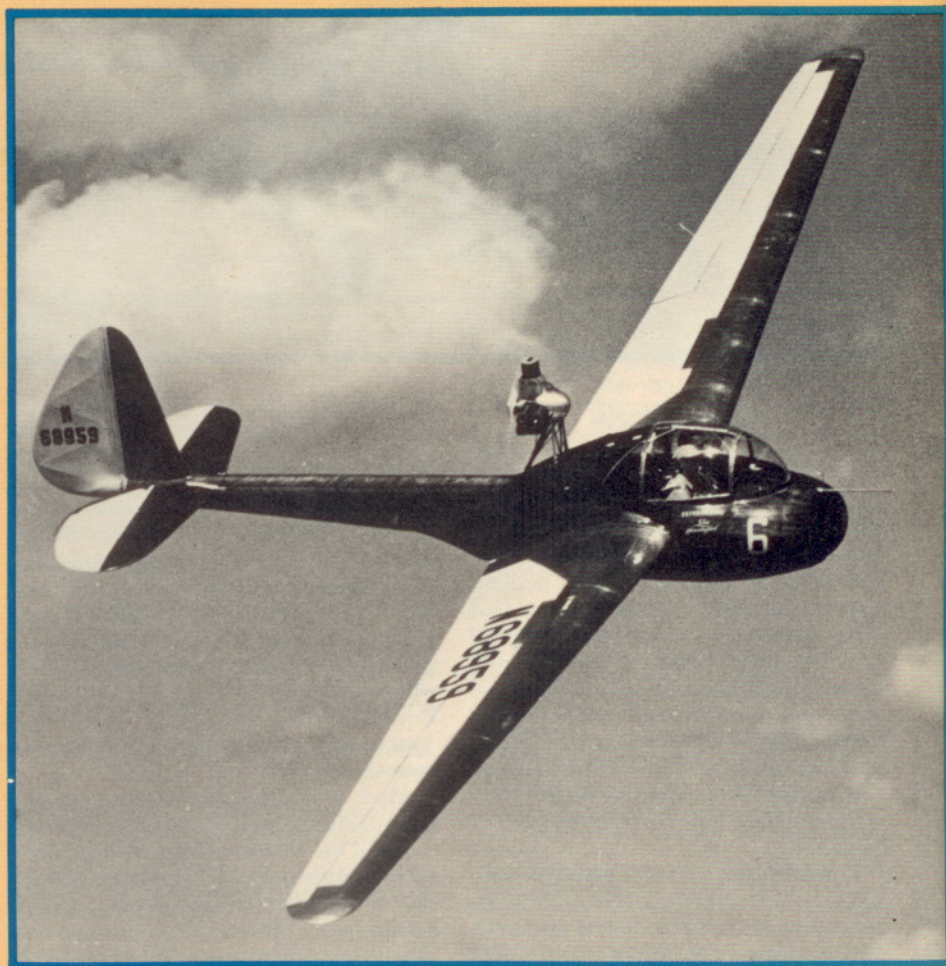
Three of the five production Nelson Dragonflies were shown in a public demonstration in Palmdale, Calif. in October 1946. Though of advanced design, the Dragonflies did not quite overcome the traditional "overweight and underpowered" handicap of previous powered gliders. Ted Nelson developed a better sailplane, the Hummingbird, with an entirely new airframe attached to a Dragonfly pod and with a top-mounted engine that retracted for streamlining into the fuselage, after engine shut-down.
